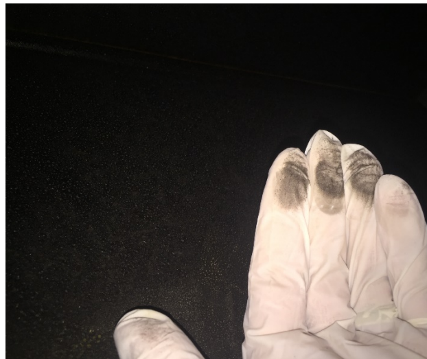
Heavy soot found inside HVAC duct in source room.
